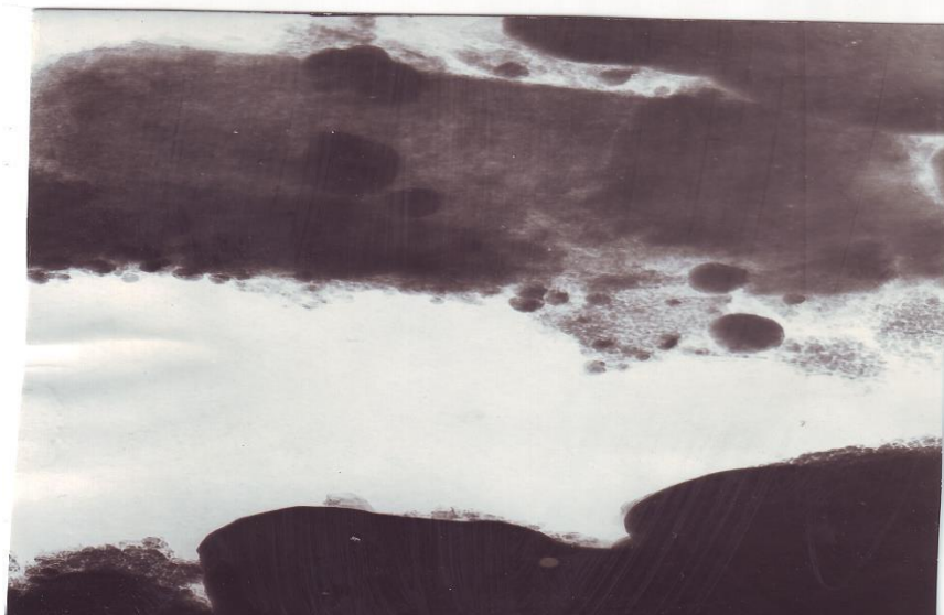
Figure-1. Electron microphotography of modified 10% Cu/ \gamma -Al 2 O 3 catalyst. (90.000x magnification)
